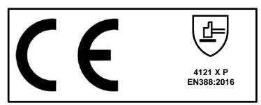
Abrasion Resistance Level: 4 of 4 Blade Cut Level: 1 of 5 Tear Resistance Level: 2 of 4 Puncture Resistance Level: 1 of 4 ISO 13997 Cut Resistance Level: X of I
