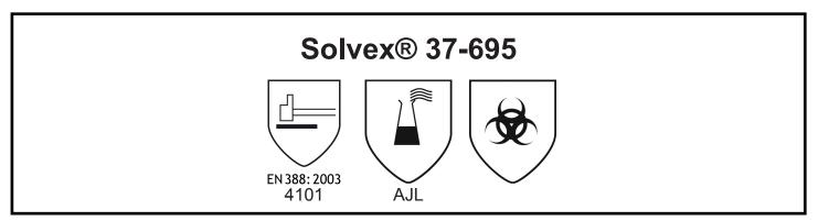
is in conformity with the provisions of the Council Directive 89/686/EEC and with the European harmonised standards EN420:2003+A1:2009, EN388: 2003, EN374: 2003, and is identical to the PPE which is subject to the EC Type Examination certificate number 3205079 issued by the Notified Body:
