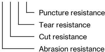
Pictogram and performance levels according to EN 388:2003 (highest performance level: 4/cut resistance: 5)
